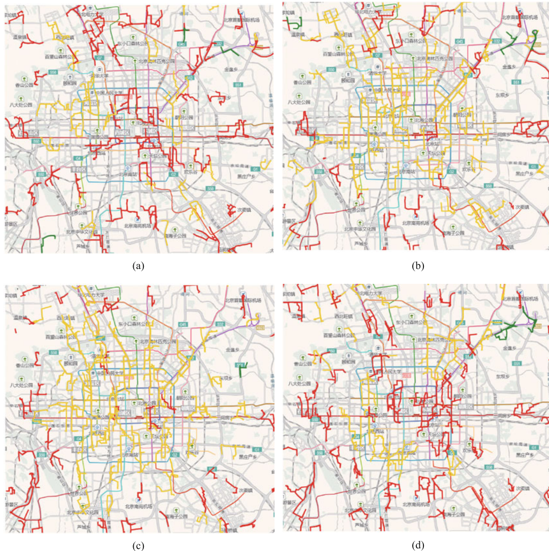
Fig. 12 Estimating mean speed of road segments in Beijing. (a) 8:00–8:30; (b) 10:00–10:30; (c) 14:00–14:30; (d) 17:00–17:30
