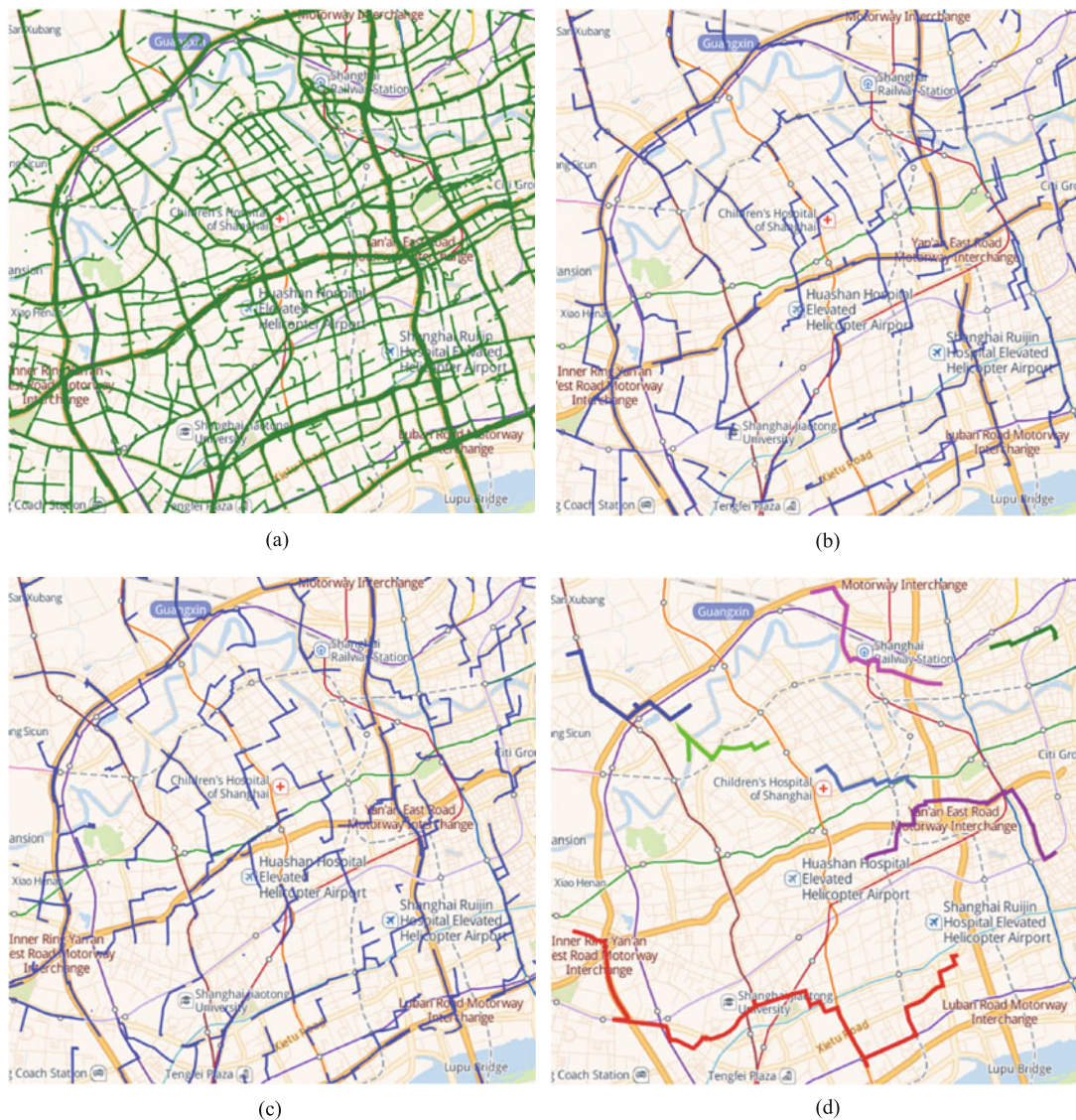
Fig. 11 Indications of high-vehicular-density route distribution in Shanghai. (a) Movement distribution within (10:00–10:30); (b) Micro-clustering within (10:00–10:10); (c) Micro-clustering within (10:10–10:20); (d) Macro-clustering within (10:00–10:30)
