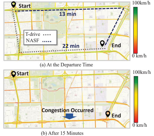
Figure 2: Visualization of traffic speed information in road networks. A darker color indicates a lower traffic speed.
