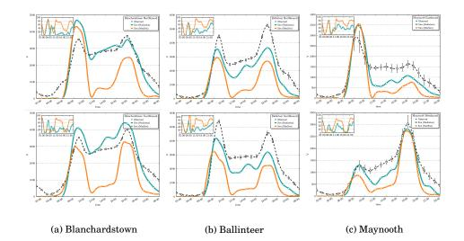
Fig. 12. Observed and simulated counts for various points around Dublin. The observed counts (dotted line) are shown with errors bars for a 24hr period. The inset shows the relative percentage error of the MATSim counts with each destination choice model.
