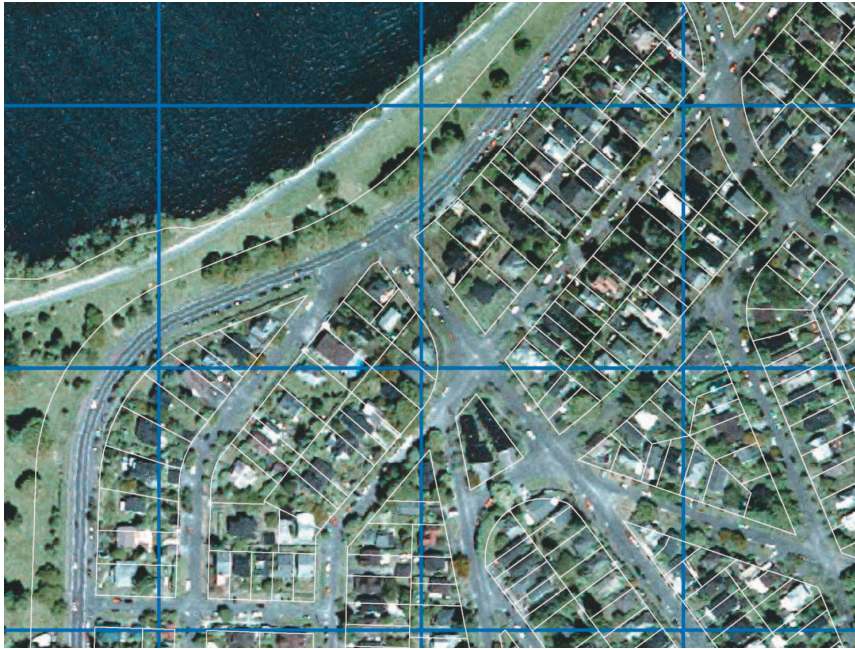
Figure 1. UrbanSim's geographic representation. The small white polygons are individual lots, while the blue squares are the 150-meter grid cells that form the core of UrbanSim's geographic representation. The data is for the Green Lake neighborhood in Seattle, Washington.
